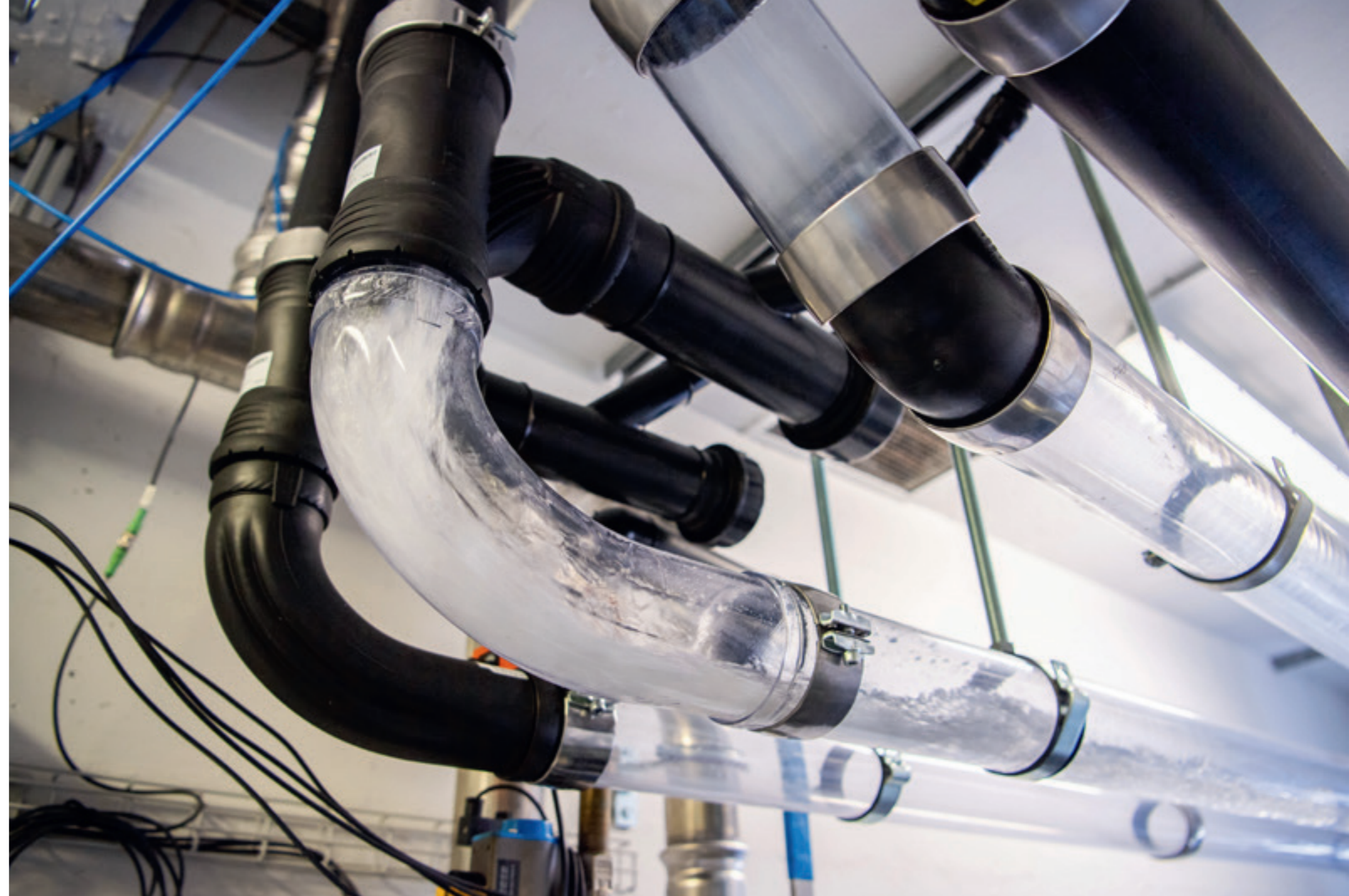
The test with transparent parts provides insights into the actual flow behaviour of the new fittings
