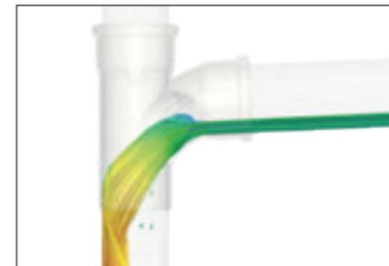
With CFD (computational fluid dynamics) numerical flow simulation, variants can be tested virtually in advance...
